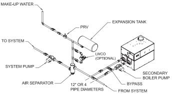
FIG. 38 Boiler with Low Temperature Bypass Piping
